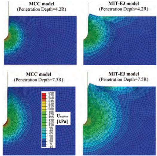
Figure 3. Excess pore pressure fields for undrained penetration in  $K_0$ -normally consolidated BBC (MCC and MIT-E3 models).
