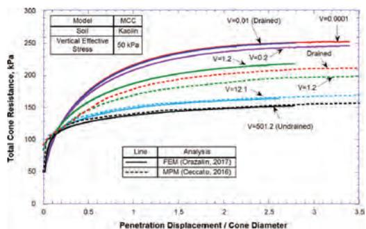
Figure 8. Comparison between proposed FE analyses and results reported using MPM method ( $\mu = 0$ ) using MCC model for NC Kaolin.
