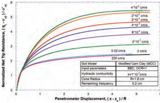
Figure 6. Effect of penetration rate on computed penetration resistance using MCC soil model.
