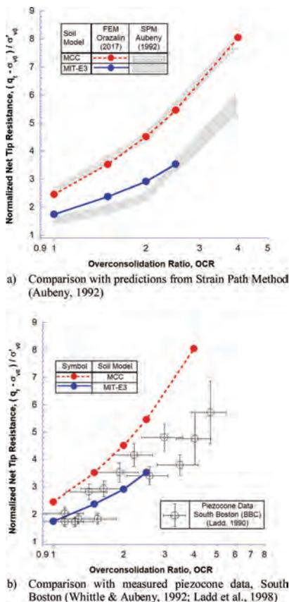
Figure 5. Evaluation of FE predictions of undrained penetration resistance in BBC.
