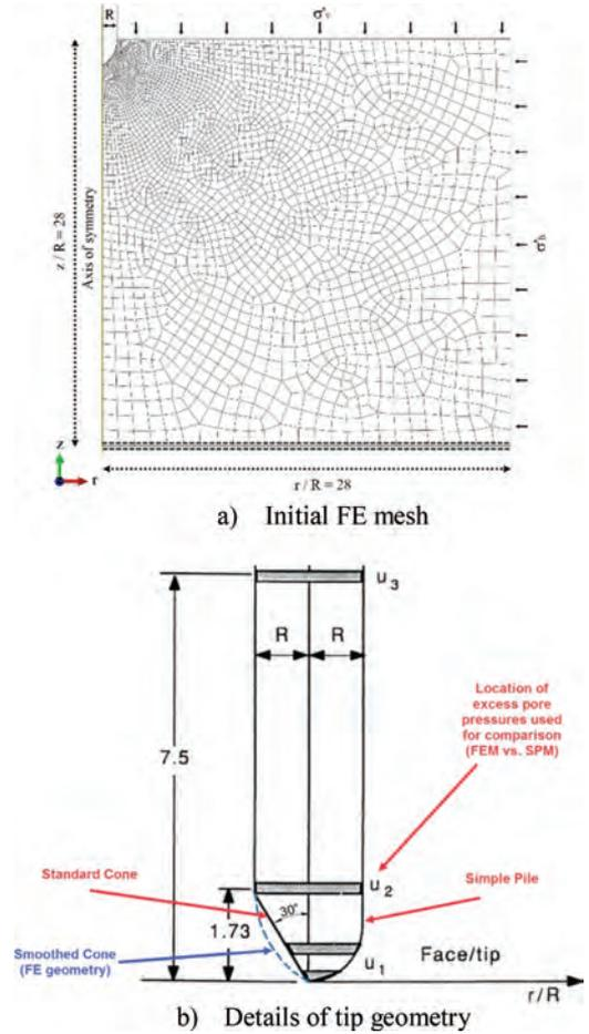
Figure 2. Finite element model of axisymmetric piezocone penetration.
