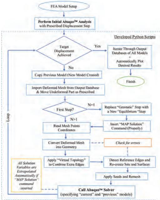
Figure 1. General algorithm for automated re-meshing and solution mapping in FE analysis (Orazalin, 2017).
