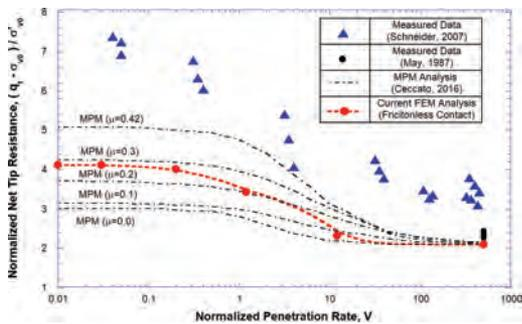
Figure 9. Comparison of computed and measured effects of partial drainage on piezocone tip resistance in kaolin.
