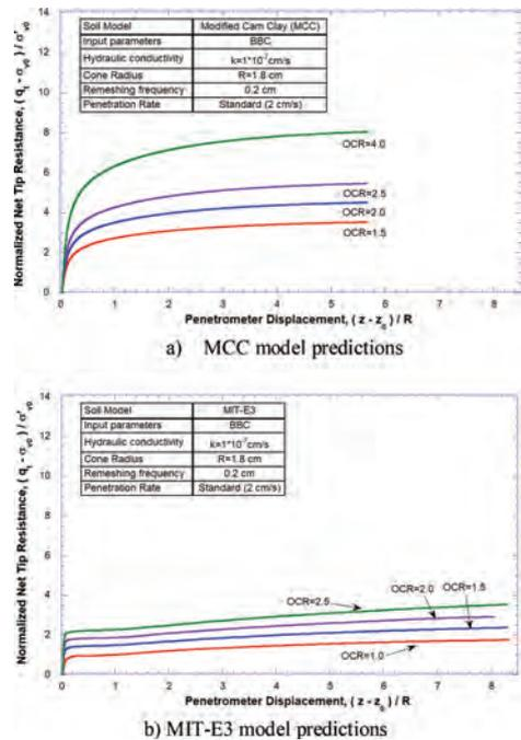
Figure 4. Effect of soil model and stress history on predictions of undrained penetration resistance.
