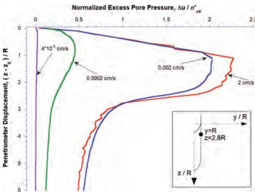
Figure 7. Effect of penetration rate on computed penetration resistance using MCC soil model.
